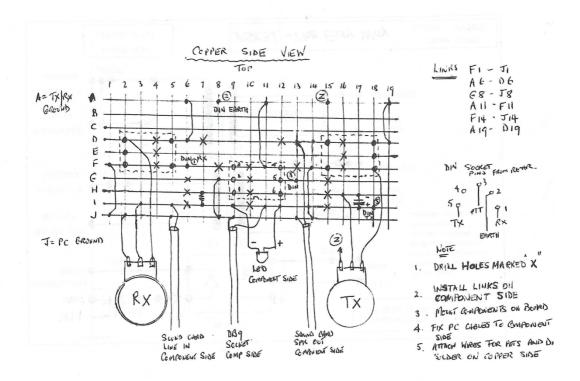
Using a small piece of vero-board and the pattern above you can build this interface in a very short time. Parts are available from Wiltronics or Jaycar.
