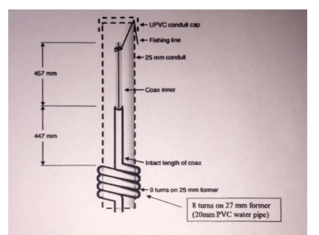
A version for 6m is also shown on the next page. Again, a modified choke is needed for water pipe instead of conduit.
