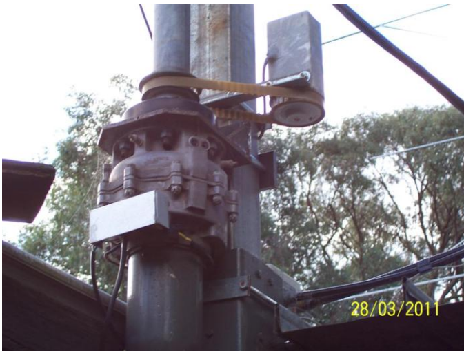
Prop Pitch Motor and Square Toothed Belt/Gear driving Azimuth Encoder
