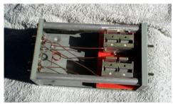
discovered the tuner doesn't work on 6m. I was told it had a fault when I got it, but had never been able to work out what that was. A bit more googling on 6m tuners, it looked like it shouldn't be too hard to make one up. With bits picked up over a few George Fowler auctions, I managed to build up a simple tuner that easily pulled the 6m antenna back to a 1:1 SWR.
