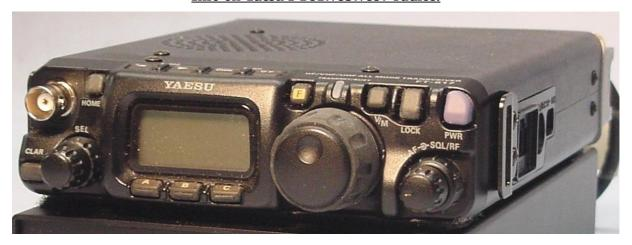
The FT817 has a fragile PA stage although the later ND model has a different and hopefully more robust design, with careful use (good VSWR) etc. not a problem.
