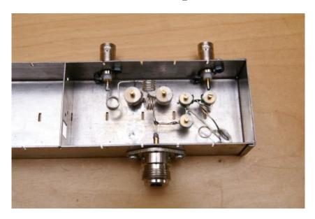
With this diplexer, you can connect a 2m (144-146 MHz) and 70cm (430-440 MHz) transmitter to a single dual band antenna, or a dual band transmitter to two separate antennas.
