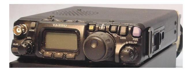
The FT817 has a fragile PA stage although the later ND model has a different and hopefully more robust design although with careful use (good VSWR) etc. not a problem.
